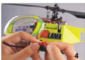
4. 连接直升机电源 Connecting the battery
